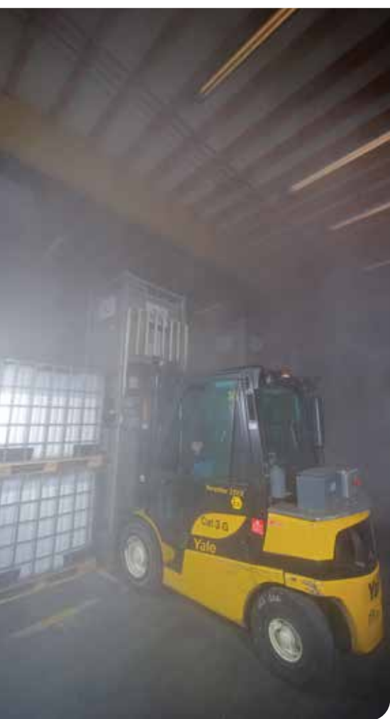
Use of explosion-proof forklifts
