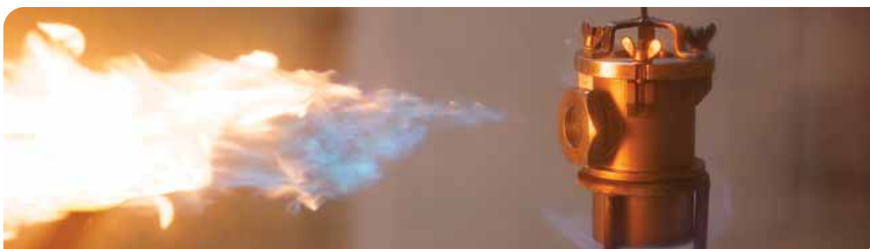
Safety testing to determine the sensitiveness of peroxides to the effect of heat under confinement
