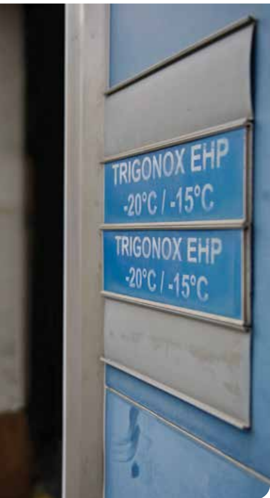
Storage temperatures near the entrance of the storage rooms
