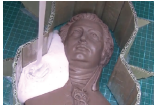
(taking care to pour the silicone away from the object to be moulded)
