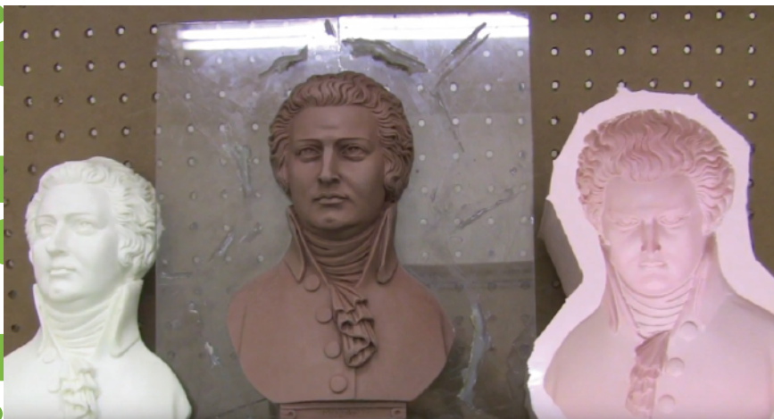
(Left: High details reproduction, Centre: Original, Right: Silicone Mould)
